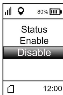
In “status” option it is possible to check if the bluetooth is enabled or disabled. Selecting “enable” the bluetooth will be activated. By selecting “Disable”, bluetooth will be disabled.
