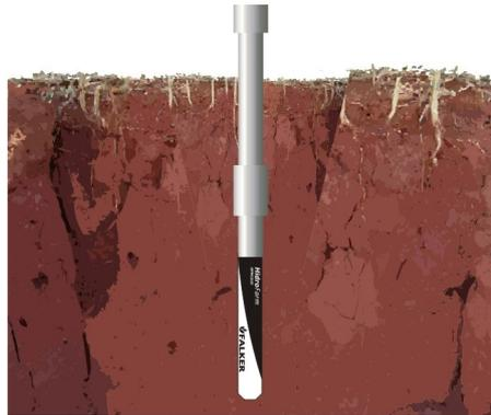
Place the cap that was used on the sensor at the end of the extender, aiming at protecting the connector.
