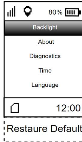
In “Backlight” option it is possible to change the intensity of the equipment screen brightness. In “About” it is possible to check information about how many measurements are stored in the memory, the battery charge level and the battery temperature. In the “Diagnostics” menu some more specific information about the battery, GPS, Memory, Sound, LEDs can be obtained.
