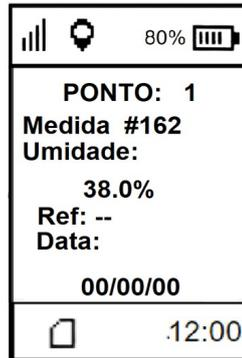
In “Measurement”, the identification of the humidity measurement carried out at the point in question is presented. In “Humidity” the humidity value of that measurement is displayed. The reference and measurement date are shown at the bottom..
