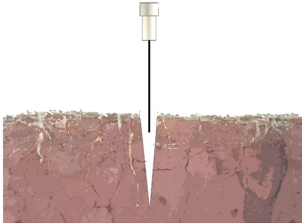
After insertion of the sensor into the created incision, the contact between soil and the sensor must be guaranteed. The best way to ensure this contact throughout the sensor is to insert a cutting blade about 20 cm away from where the sensor was installed on both sides and press the ground towards the sensor.
