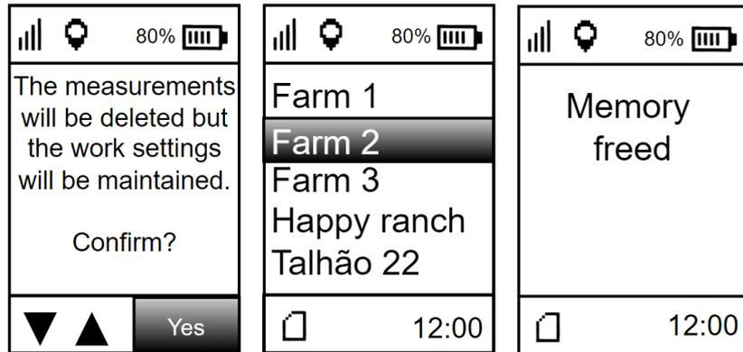
By choosing the “delete work” menu, it is possible to delete the entire structure of a previous work. The first screen that opens tells you what the operation will do and requires confirmation to proceed. On the second screen, the work to be deleted must be chosen. The last screen is confirmation that the action was done correctly.
