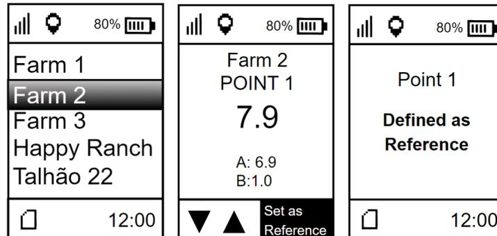
By clicking on the “Add work” menu, the screen for choosing the name of the new work will open. To choose the letters, use the directional arrows. To confirm the letter, use the enter key. After choosing the name, the screen for choosing the number of points that will compose the new work is opened. Finally, it is necessary to choose the number of measurements that will be part of each point. The figure 16 below shows the chaining of screens in the “Add work” menu.
